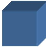
$$\frac{\Delta V_x}{V} = \frac{\Delta V_y}{V} = \frac{\Delta V_z}{V} = \alpha_a T \rightarrow \frac{\Delta V_{ges}}{V} = 3 * \alpha * \Delta T \Rightarrow \gamma = 3\alpha$$
